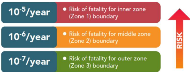
Figure 4 Individual risk zones to be plotted on a map according to the guide [2]
