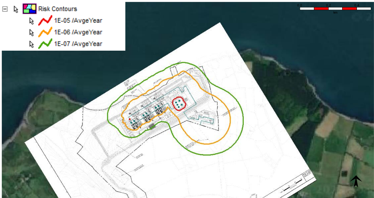
Figure 12 Outdoors Individual Risk Contours with plot plant
