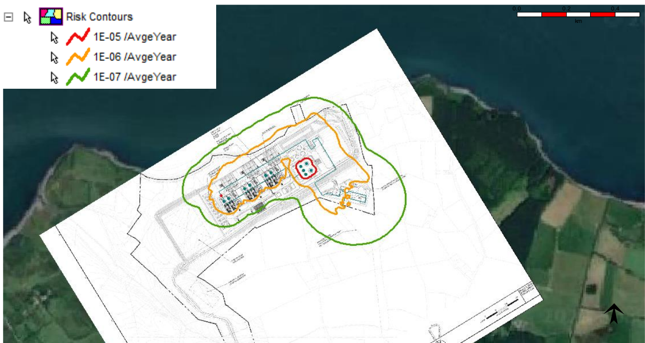
Figure 14 Indoors Individual Risk Contours with plot plant
