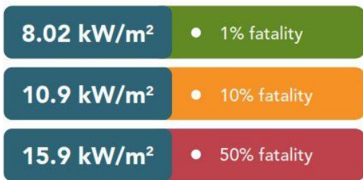
Figure 6 Heat flux and fatality levels, outdoor, for a 60s exposure
